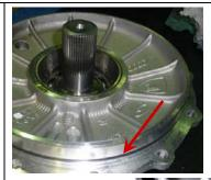
Lubricate the screws with Loctite® 242 and Medio thread sealant. Tighten the screws to 35Nm, as shown in the sequence in the photograph.
