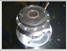
Extract the planetary gear to be replaced and the friction disk pack.
